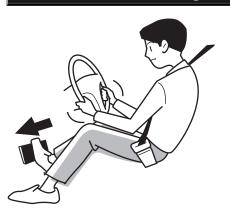
As the brake booster will no longer operate, brake effectiveness will be reduced. The power steering system will not work so the steering wheel will be hard to turn. Stay calm and decrease vehicle speed by depressing the brake pedal. Then, promptly pull the vehicle over to a safe location and inspect its condition. If the engine does not start, contact the nearest Isuzu Dealer.
