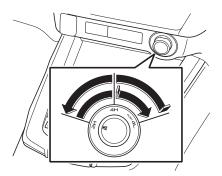
Use the 4WD switch to select 2WD or 4WD ("4H (4WD high)" or "4L (4WD low)").
