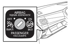
The passenger side SRS airbag on-off switch is positioned below the instrument panel on the passenger side. Open the glove compartment to check the switch. Always ensure that the passenger side SRS airbag on-off switch is in the proper position before driving.
