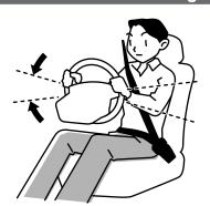
While the engine is idling, place the steering wheel in the straight forward position, then gently turn it to the left and right by hand, and check the play in the steering wheel as the peripheral distance to the point where the tires start moving.
