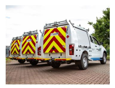
Equipping the truck to Western Power's exact specification, Isuzu's Fleet Services team installed a speed limiter and a 'Scorpion' alarm, which had been extended to protect both the vehicle and body conversion. In addition to building and fitting the body, Strongs also designed and fitted a drawer system with push-button retainers, roller shutters, a 1000W inverter, Chapter 8 decals, Tow Trust rear steps, magnetic work lamps and more.
