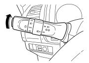
Turning the light control switch to the position indicated in the table causes the relevant lights to illuminate.
