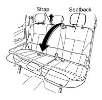
It is possible to fold the seatback forward by pulling the strap.
