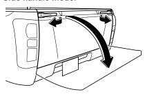
Pull the handle on both sides of the tailgate and release the lock. Open the tailgate slowly.
