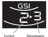
The GSI assists in gear selection to enable improved fuel economy when driving. In addition to displaying the current gear position on the instrument panel, it also displays the recommended gear position when there is a gear in which fuel economy would be improved. The GSI display can be switched between the following 3 patterns.
