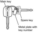
Both sides of the key are identical, so you can insert the key in the key cylinder without worrying about which way you insert it.
