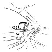
Lateral-direction: Adjust the mirror so that you can see the vehicle's side including the inner one-third of the mirror.
