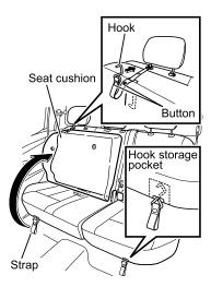
Pull the strap forward to raise the seat cushion. Remove the hook of the strap edge from the strap button and secure the hook to the headrest stay.
