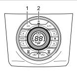
3. To turn off the air conditioning system, press the A/C switch (2). To turn off both the fan and air conditioning system, press the OFF switch (1).
