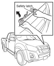
Insert a hand with its palm facing down into the space under the front edge of the engine hood, push the safety latch leftward to release the lock, and open the engine hood.
