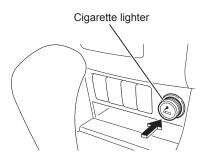
The cigarette lighter can be used when the power mode is "ACC" or "ON" (models with passive entry and start system) or the starter switch is in the "ACC" or "ON" position (models without passive entry and start system).
