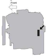
The engine number is stamped on the left side rear part of the engine block.
