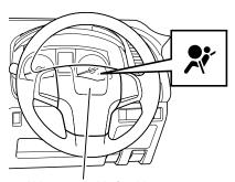
Airbag assembly for driver seat
