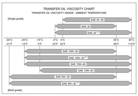
\*1: Use is possible at ambient temperatures up to 45°C (113°F) only in the case of Isuzu genuine oil.
