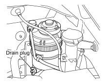
The fuel filter is located at the rear left side of the engine compartment.
