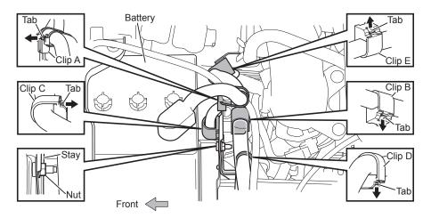
7. Loosen the nut and remove the stay.
