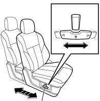
Fore-aft position and height adjustment lever
