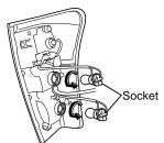
3. Pull out the bulb from the socket.
