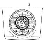
Press the AUTO switch (3). The air conditioning system will turn on, and automatically select the air outlets and fan speed most suitable for the condition of the interior of the cab. The display will then show "AUTO".
