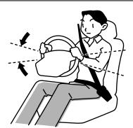
While the engine is idling, place the steering wheel in the straight forward position, then gently turn it to the left and right by hand, and check the play in the steering wheel as the peripheral distance to the point where the tires start moving.
