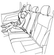
Use this type of restraint system when children outgrow a typical front-facing CRS but they are still too small for lap/sash seat belts. A booster seat raises the child so that the knees bend comfortably, the lap /sash seat belt is correctly positioned and the child can see out the window. A rigid booster seat with a back, side wings and sash guide gives the best protection. In assessing the range of children who would benefit from booster seats, height is a better indicator than age or weight.
