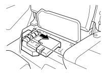
Loosen the jack release knob to remove the jack. Slide the cover of the emergency flat tire repair kit sideways, then pull out the emergency flat tire repair kit.
