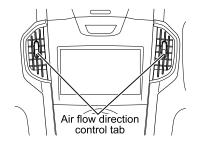
Use the tab to control the air flow direction from the outlet. To close the outlet, move the tab fully down.
