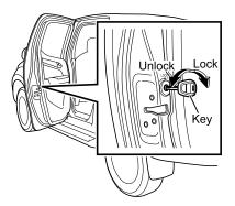
Use the locks if you are traveling with a child in the vehicle. Use the key for the child-proof function of the opening of the rear door, place it in the "LOCK" position and close the door. Regardless of the position of the lock knob, it will no longer be possible to open the rear door from inside the vehicle.
