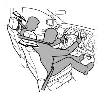
When the vehicle receives an impact exceeding a certain level during a frontal collision, or lateral collision (in models with side airbag and curtain airbag), the fastened seat belt is retracted instantly and removes the slack in the seat belt to securely restrain the driver and the passenger in the seat, thus enhancing the seat belt's restraining effect.
