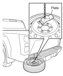
1. Set the disc wheel so that its outer surface faces up, and then insert the plate into the center of the disc wheel.
