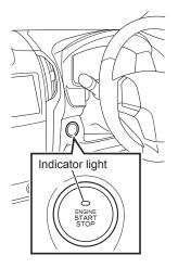
This button is used to start/stop the engine and switch the power mode.
