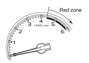
The tachometer indicates the engine speed in revolutions per minute (r/min). (Graduation "1" on the scale indicates 1,000 r/min.) The red zone indicates a range of dangerous engine speeds beyond permissible levels.
