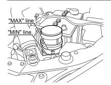
The reserve tank is located at the front of the engine compartment on the left. The fluid level is correct if it is between the "MAX" and "MIN" lines on the reserve tank. If the level is lower than the "MIN" line, add power steering fluid up to the "MAX" line. Furthermore, perform an inspection for power steering fluid leaks.
