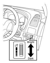
This switch is used to adjust the brightness of the illumination in the instrument panel. Turning the switch up brightens the lights, and turning the switch down darkens them. The brightness can be adjusted with the light control switch in the "\_OO\_" or " O" position.
