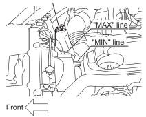
When the engine coolant level in the reserve tank is below the "MIN" line, open the tank cap and fill to near the "MAX" line with engine coolant. Tighten the cap securely after the engine coolant has been replenished.
