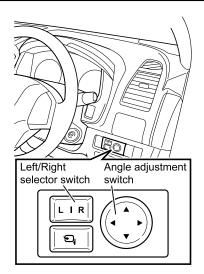
The remote control mirror switch is active only when the power mode is "ACC" or "ON" (models with passive entry and start system) or the starter switch is in the "ACC" or "ON" position (models without passive entry and start system).
