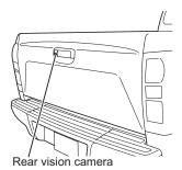
The rear vision camera is installed to the tailgate.
