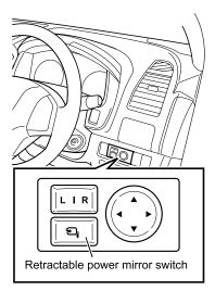
The retractable power mirror switch is active only when the power mode is "ACC" or "ON" (models with passive entry and start system) or the starter switch is in the "ACC" or "ON" position (models without passive entry and start system).
