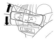
When turning left or right, move the lever up or down to flash the turn signal light.
