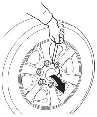
4. For models with aluminum wheels (except for 18-inch), remove the wheel cover using a flat-head screwdriver or flat end of the jack handle. Insert the driver or the jack handle into the hole and pry the wheel cover off.
