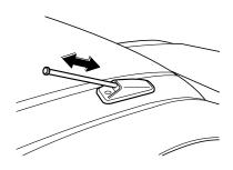
When receiving radio signals, pull the antenna out by hand to extend it to its full length.
