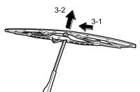
With the blade and arm almost perpendicular, remove the blade from the arm.
