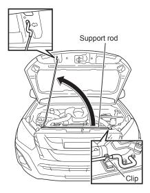
Remove the support rod from the clip, and then install the support rod edge hook into the groove of the engine hood.
