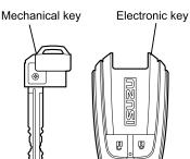
The passive entry and start system is a system that enables doors to be locked and unlocked and for the engine to be started remotely just by carrying the electronic key in your pocket.
