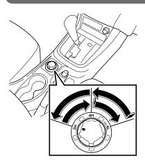
Use the 4WD switch to select 2WD or 4WD ("4H (4WD high)" or "4L (4WD low)").
