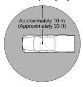
The passive entry and start system and keyless entry system (radio remote control units for door-lock) allow you to lock/unlock the doors by simply pressing the button on the remote control unit without inserting the key into the lock.
