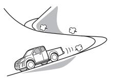
When driving down a long slope, use engine brake together with the foot brakes. Using the low-gear engine brake reduces the work load on the foot brakes and yields greater braking force. In automatic transmission models, do not use the auto mode, as it does not provide engine efficiency. Use only the manual mode for engine braking.
