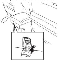
The USB power outlet can be used when the power mode is "ACC" or "ON" (models with passive entry and start system) or the starter switch is in the "ACC" or "ON" position (models without passive entry and start system).
