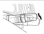
Windshield washer fluid is sprayed over the windshield when this switch is pressed. At the same time, the windshield wiper operates.
