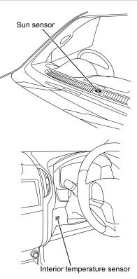
The air conditioning system uses a sun sensor, interior temperature sensor and outside air temperature sensor to ensure effective and comfortable air conditioning. Do not place anything on the sensors or get them wet. Air conditioning control will become inaccurate.
