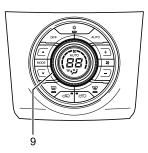
Use the temperature control dial (9) to set the interior temperature to the preferred level. The display will show the set temperature. Each turn of the dial by one notch changes the temperature by 1°C (1.8°F).
