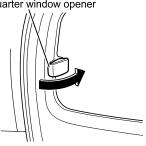
The quarter window on each side can be opened and closed by operating the quarter window opener.
