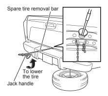
Insert the spare tire removal bar into the hole in the spare tire carrier, and turn the jack handle counterclockwise to remove the spare tire.
