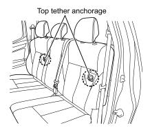
Top tether anchorages are installed on the panel behind the rear seats.
