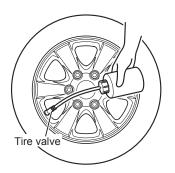
5. Hold the sealant bottle with the bottom upward and pump the sealant bottle to fill the entire contents of the sealant bottle into the tire. After filling the entire contents of the sealant bottle into the tire, pull off the filler hose. Firmly screw the valve insert into the tire valve.
