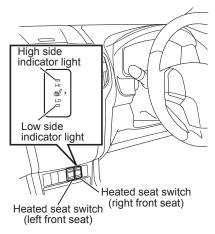
The heated seat can be used when the power mode is "ON" (models with passive entry and start system) or the starter switch is in the "ON" position (models without passive entry and start system).
