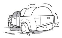
When driving in sand or mud, go as slowly as possible, avoiding hard braking, sudden acceleration and sharp turns of the steering wheel.
