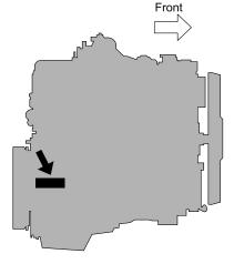
The engine number is stamped on the right side rear part of the engine block.
