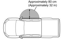
By carrying the electronic key, it is possible to lock or unlock the doors by operating the lock button or door handle on the driver side door. The key must be within approximately 80 cm (32 in) of the driver side door handle, in order to lock or unlock the doors.
