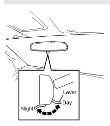
Normally, with the lever pushed toward the front of the vehicle, move the mirror to adjust to a position where it provides a proper rear view. When the headlights of vehicles behind you are reflected brightly when driving at night, pull the lever toward you. By doing this you can reduce the reflection.
