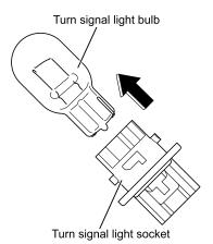
3. Pull out the bulb from the socket.
