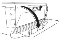
Pull the handle in the center of the tailgate and release the lock. Open the tailgate slowly.
