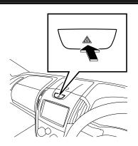
The hazard warning flasher is used to signal other vehicles that your vehicle is stationary on the road because of an accident or component failure.
