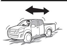
If the vehicle gets stuck in mud, pressing the accelerator pedal more than necessary will simply dig the vehicle deeper into the mud and make it harder to extricate. Either put stones, tree branches or blankets under the tires to gain traction or repeatedly drive forward and backward to use the vehicle's momentum to extricate it.
