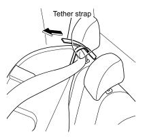
8. Adjust the tether strap length until it attached tightly with the seat structure.
