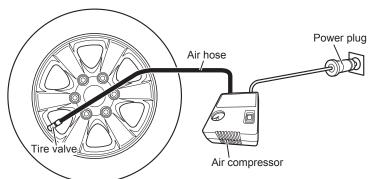
6. Screw the air hose of the air compressor into the tire valve to connect them. Install the power plug to an accessory power outlet. Turn the starter switch to the "ACC" position and turn "ON" the air compressor power. Fill the tire to the specified air pressure.
