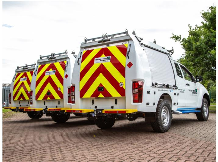
Equipping the truck to Western Power's exact specification, Isuzu's Fleet Services team installed a speed limiter and a 'Scorpion' alarm, which had been extended to protect both the vehicle and body conversion. In addition to building and fitting the body, Strongs also designed and fitted a drawer system with push-button retainers, roller shutters, a 1000W inverter, Chapter 8 decals, Tow Trust rear steps, magnetic work lamps and more.
