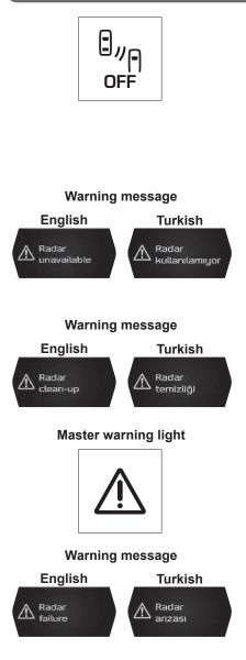
When the blind spot monitor (BSM) is turned off by using the user customization function on the MID, the BSM OFF indicator light on the instrument panel comes on. This indicator light also comes on in the following cases.
