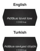
This message appears on the display for 5 seconds if the AdBlue<sup>®</sup> level becomes low and the remaining driving distance until the engine cannot be restarted becomes less than 2,400 km (1,491 miles).
