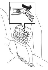
The USB power outlet can be used when the power mode is "ACC" or "ON" (models with passive entry and start system) or the starter switch is in the "ACC" or "ON" position (models without passive entry and start system).
