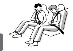
The seat belt with pretensioner and the supplemental restraint system (SRS) airbag system operate when the vehicle is subjected to an impact exceeding a certain level when a collision occurs.
