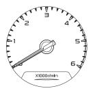
The tachometer indicates the engine speed in revolutions per minute (r/min). (Graduation "1" on the scale indicates 1,000 r/min.) The red zone indicates a range of dangerous engine speeds beyond permissible levels.
