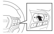
When the brake pedal is released and the SET switch or RES switch is pressed, the vehicle restarts driving at a constant speed or following the preceding vehicle according to the originally set vehicle speed. The adaptive cruise control indicator light comes on green.
