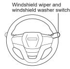
The windshield wiper and windshield washer switch is located at the position shown in the diagram.
