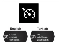
This indicator light comes on white when the cruise control main switch is pressed. This indicator light comes on green when the cruise control set switch is pressed. For models with the stereo camera, when the cruise control is canceled automatically by the system, this indicator light changes from green to white after "Cruise control canceled" is displayed on the MID for approximately 5 seconds. For models without the stereo camera.
