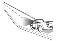
Under the following road conditions or conditions of your vehicle, the stereo camera may not be able to detect the preceding vehicle. Vehicles in neighboring traffic lanes or roadside objects may also be incorrectly detected. Under conditions such as these, do not use the adaptive cruise control. If cruise control is currently in use, operate the brake pedal and take other actions as necessary.
