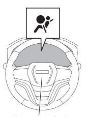
Airbag assembly for driver seat
