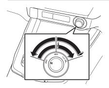
Use the 4WD switch to select 2WD or 4WD ("4H (4WD high)" or "4L (4WD low)").
