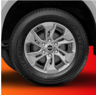
18" Alloy Wheel in Standard Silver Finish 18"X7.5J-33 265/60R18 110H: A/T Pattern AT31 [Dunlop]
