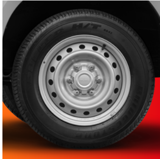
18" Steel Wheel 18"X7.5J-33 265/60R18 110H: A/T Pattern AT31 [Dunlop]
