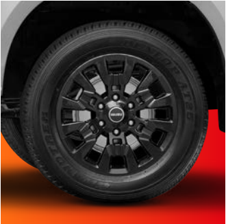
18" Alloy Wheel In Matt Dark Grey Metallic Finish 18"X7.5J-33 265/60R18 110H: A/T Pattern AT31 [Dunlop]
